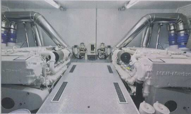
Below: This yacht was equipped with the standard engines, 900-hp MANs; 1,100-hp ones are available as an option. Right: The Navetta's wheelhouse was eerily quiet while we were underway.
